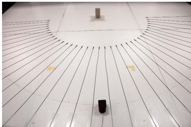
Figure 2. RPG 2D Goniometer with speaker at normal incidence, 37 receiving microphones at 5 degree intervals and a test sample of a QRD. Speaker radius is 2 m and microphone radius is 1 m.
