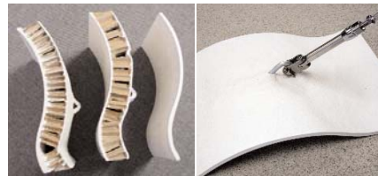
Figure 3. Three spline samples with different construction and surface weight. Left: 1 5/8" GHG 5 lbs/sf.; 1 5/8" GHG 4 lbs/sf.; 1/4" GRG 3 lbs/sf. Right: Spline with mounting cable attached
