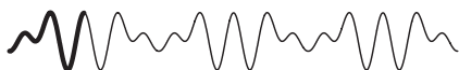
Figure 1. A 1D Waveform Spline canopy. The asymmetric base shape is shown in bold. By changing the orientation, it is possible to increase the length of the diffusor to improve uniformity of diffusion.
