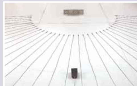
Figure 3. RPG 2D boundary plane goniometer. Impulse responses at 5 degree increments backscattered from the sample, located at the origin of the microphone and speaker semicircles, are automatically measured under computer control.
