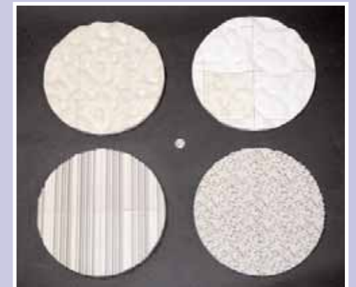
Figure 7. 1:10 scale 300 mm circular model samples of the Waveform 8'' Bicubic (top left), Waveform 4'' Bicubic (top right), Skyline (lower right) and Modffusor (lower left).
