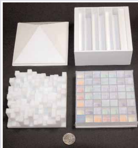
Figure 2. 1:5 Scale models. Top left: Golden Pyramid, Top right: Modffusor, Bottom left: Skyline, Bottom right: Omniffusor
