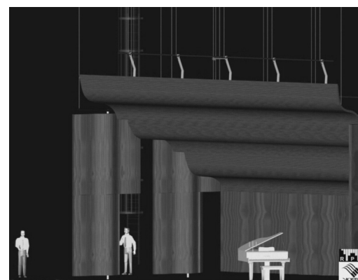
Figure 2. Overture in play position. Canopy elements are lowered and tilted. Rear wall is lowered. Side towers are lowered and rotated into position. Access doors are open.
