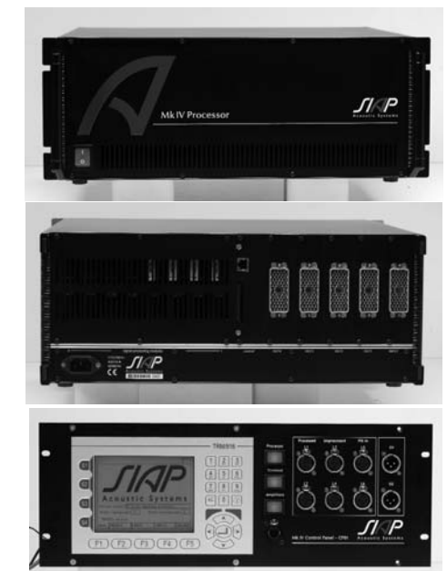
Figure 4. Top: 64 output system. Top: SIAP MKIV front panel; Middle: SIAP MKIV rear panel, showing 5 EDAC input and output connectors; Bottom: New keypad selector and input connectors.
